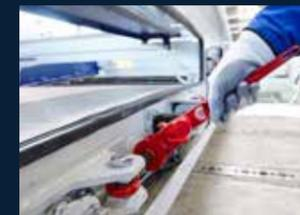
The screen cloth is tensioned once again with quick-action fasteners.
