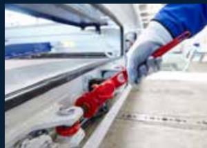
The screen cloth is tensioned by rapid-action fasteners.
