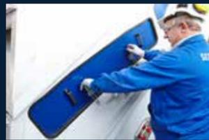
The maintenance doors at the defective screen cloth are opened on both sides.
