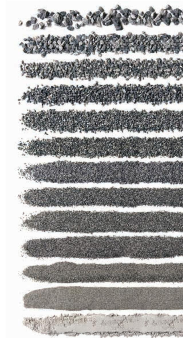
The figure to the right shows an example particle size distribution of typical FineLine feed material.
